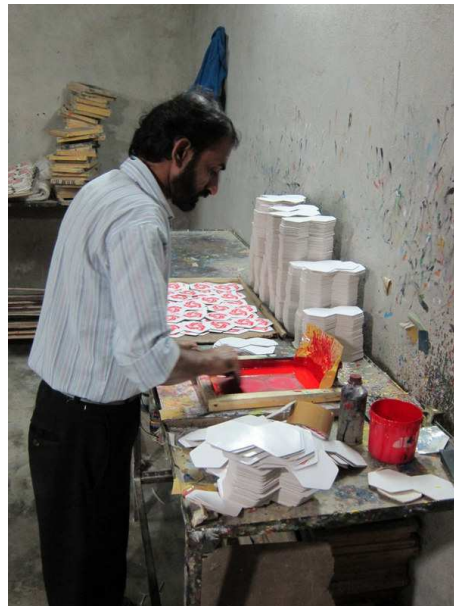
Figure 4: Printing the Designs (Step 3)
