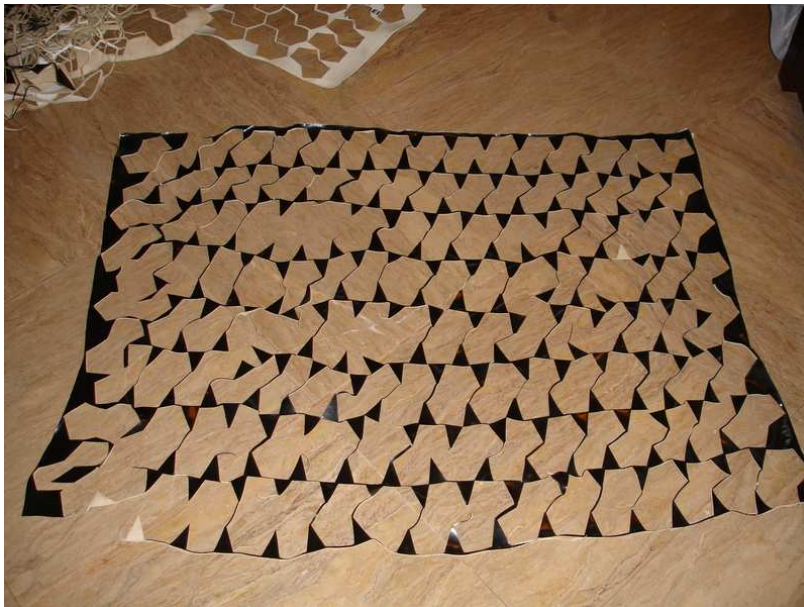
Figure 8: Laminated Rexine Wastage from Cutting Pentagons
