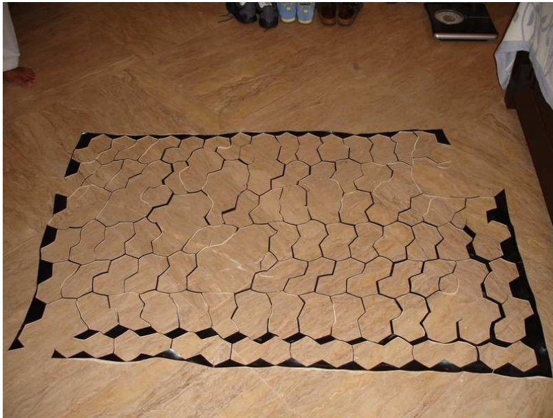
Figure 7: Laminated Rexine Wastage from Cutting Hexagons
