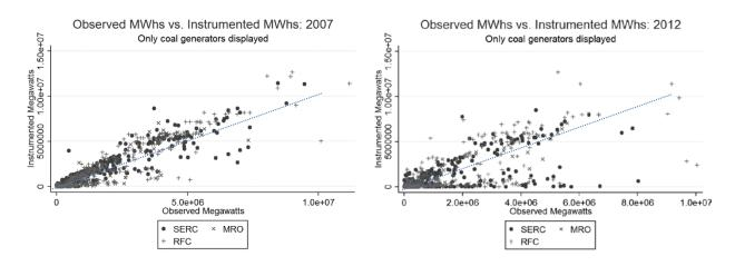
Note: 2007 and 2012 instrumented hours from dispatch model (y-axis) against observed generation in CEMS data (x-axis). Capacity measure constructed from max average hourly generation observed within a day conditional on boiler generating. Color indicates NERC region. Only coal generation displayed. 45 degree line indicated by dotted line.
