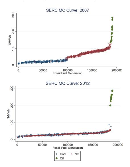
Note: 2007 and 2012 constructed SERC supply curves. Data are taken from CEMS and SEDS datasets. Capacity measure constructed from max average hourly generation observed within a day conditional on boiler generating. Red dots represent natural gas-fired capacity; the 2012 curve displays significantly more mixing at lower levels of generation.
